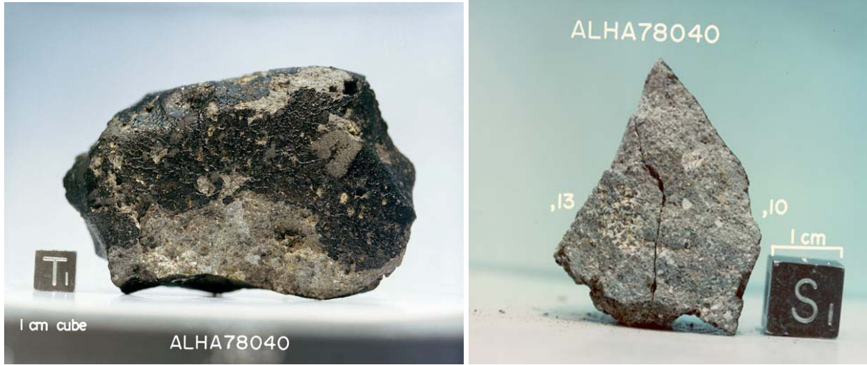
Figure 21: Laboratory images of ALH A78040 in the meteorite lab at NASA-JSC. The left-hand image shows the fusion crusted exterior (NASA photo S79-33368). The right-hand image shows the interior with a prominent basaltic clast to the left of the vertical fracture (NASA photo S80-26737). Both images have a 1 cm cube for scale.
