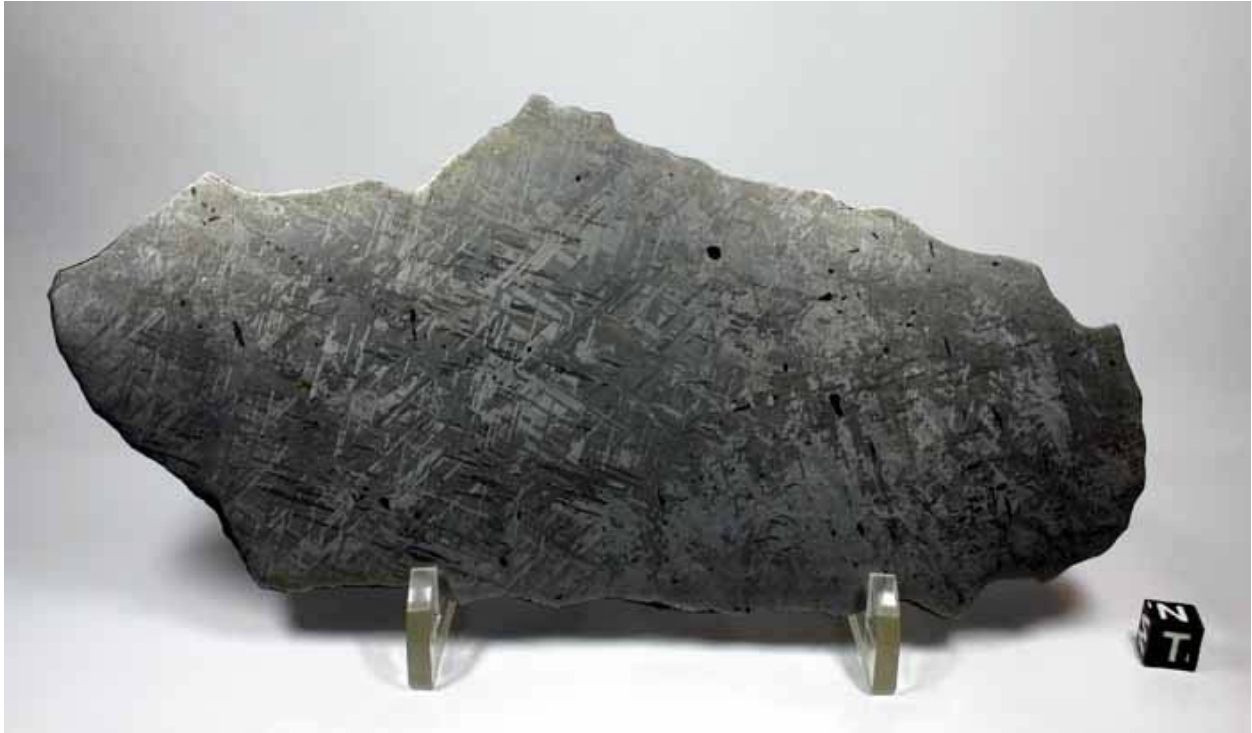
Figure 28: An etched surface of a slice through the Gibeon iron meteorite; 1 cm cube for scale.
