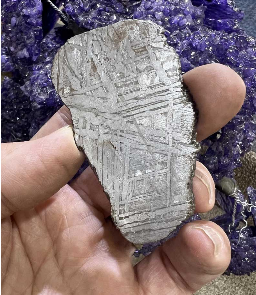
For the smaller taste, an elegant etched hand specimen of Muonionalusta provides an abundance of octahedrite crystal faces to gaze at.
