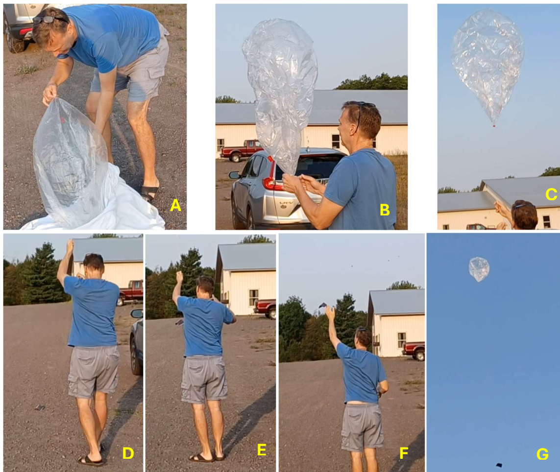
Figure 10. Launching the tracker. A. Remove the balloon from the sheet and remove the weights. B. Hold the balloon by the attachment point until the wind is low. C-E. Let the balloon rise as you walk toward the tracker. F. Release the line when the tracker is at head height. G. Liftoff!
