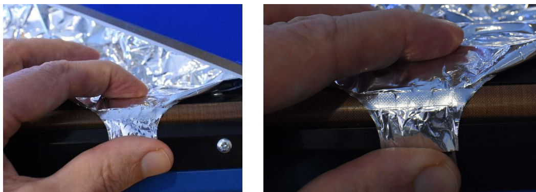
Figure 4. Sealing the balloon stem with an impulse sealer
