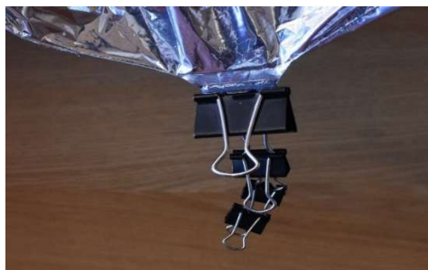
Figure 2. Payload simulation weights attached to balloon
