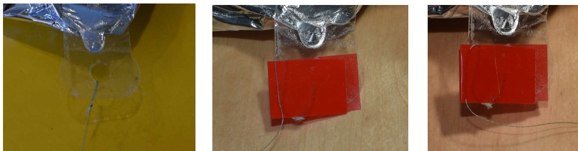
Figure 6. Attaching the balloon payload line
