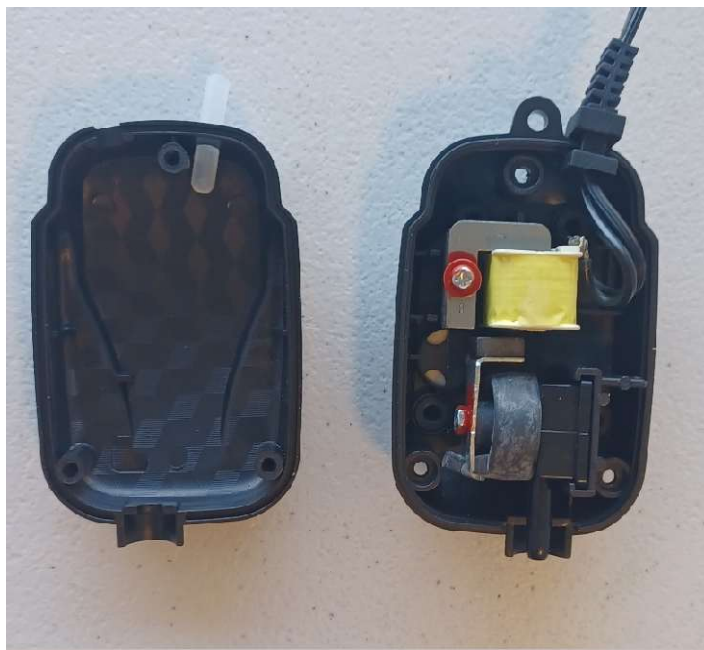
Figure 1. Modified Aquarium Pump
