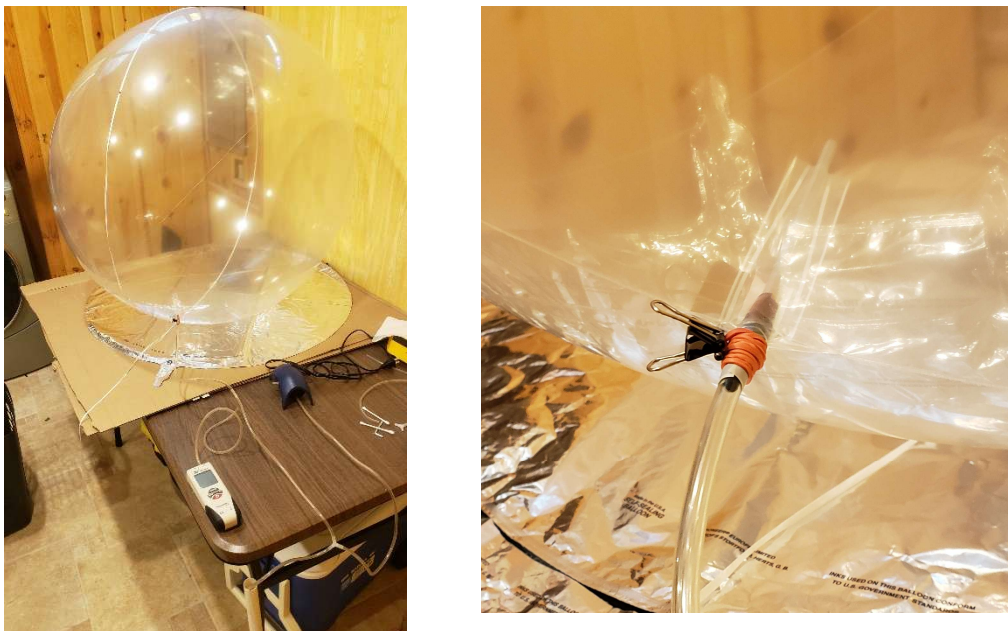
Figure 4. Stretched Balloon and view of internal self-sealing fill stem
