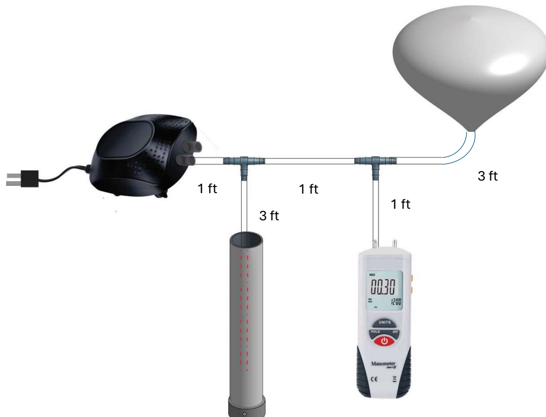
Figure 2. Balloon stretching system
